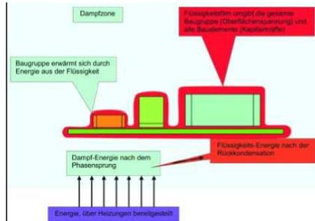
Image 2 Energy flow in a vapor phase
