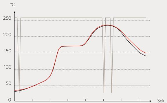
Multi Vacuum Technology enables up to three vacuum steps per soldering cycle.
